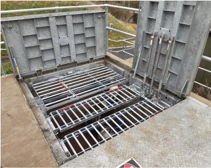
Fall protection safety grids and covers fitted with 3 mechanical struts for lift assistance. Safety stay bars are a standard feature to prevent covers from freely closing.
